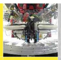
The system provides significant productivity advantages in terms of manufacturing speed as well as overall panel weight reduction of about 15% vs the traditional riveting process.
