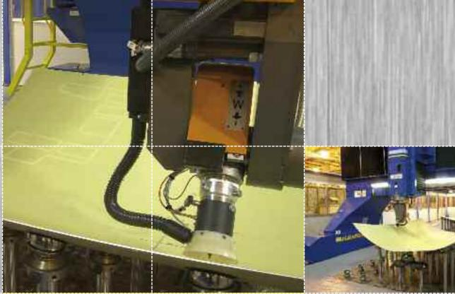
By integrating the TORRESTOOL® with the TORRESLASER<sup>®</sup> 5 axes High Speed Laser Machine, the system provides the highest degree of flexibility and reduces changes over time from one work piece configuration to another to less than 2minutes. All supports rods with vacuum cups move simultaneously in the X/Y/Z axes and are automatically locked in their final positions.
