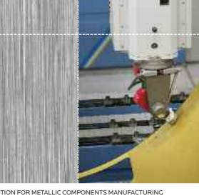
**TORRESLASER® 5-axes** gantry DNC-CNC high speed Laser machine series has been specially designed for high speed laser Maskant cutting for chemical milling process of aircraft Aluminium structural components. The TORRESTOOL<sup>®</sup> provides the maximum flexibility.
