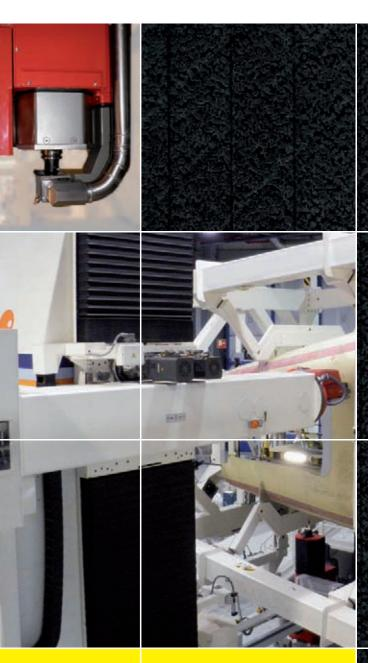
By integrating the TORRESTOOL<sup>®</sup> with the TORRESDRIL, the system provides the highest degree of flexibility. All supports rods with vacuum cups or clamping devices move simultaneously in the X/Y/Z axes and are automatically locked in their final positions. The TORRESDRILL Automatic Drilling and Countersinking Machine specially designed for high speed drilling and countersinking Carbon Fiber components, as well as stacks of different materials.
